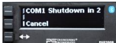
Figure 3-4 COM 1 Shutdown message
